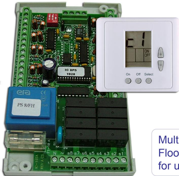
Multi-zone main controller for Floor Heating applications, for up to 8 rooms.
